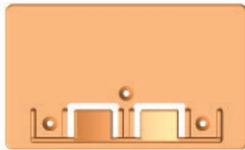
**STEP 2** Fit base into bottom bracket and screw top of unit (marked x) to wall using wall plugs as required, or optional bracket.
