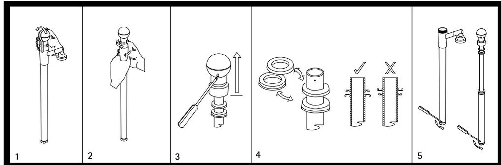
**Should the Drumpump fail to pump replace the valve flaps. Ask for Ezi-action® Service Kit (Refer Steps 5-9)**
